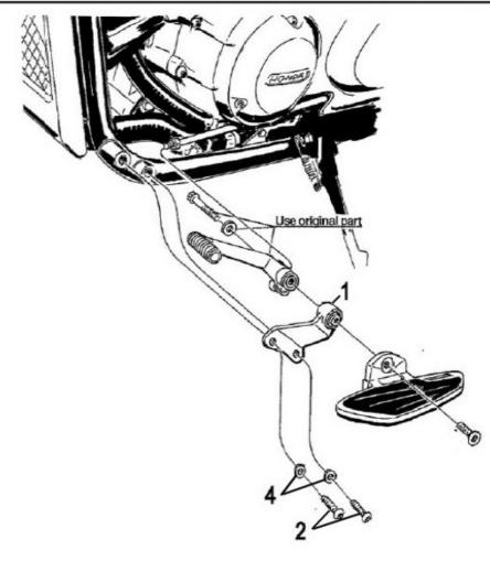
Please check all fixings and mounting points before assembly as listed on the mounting instrucion sheet.
